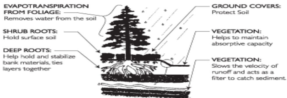
FIGURE 1. ROLE OF VEGETATION IN REDUCING EROSION AND STABILIZING SLOPES. (MENASHE, 1993)
